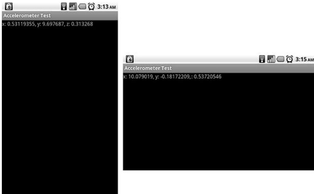
Figure 4-9. Accelerometer axes' values in portrait mode (left) and landscape mode (right) when the device is held perpendicular to the ground
