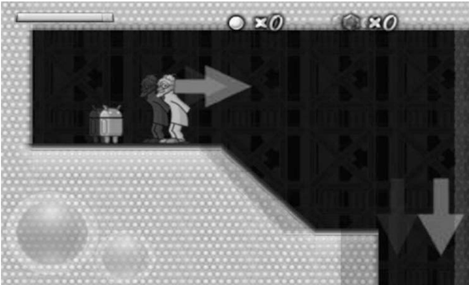
Figure 5-2. Replica Island stretched from 480×320 to 800×480 pixels, overlaid with a faint image of how it is rendered on an 800×480-pixel display without stretching
