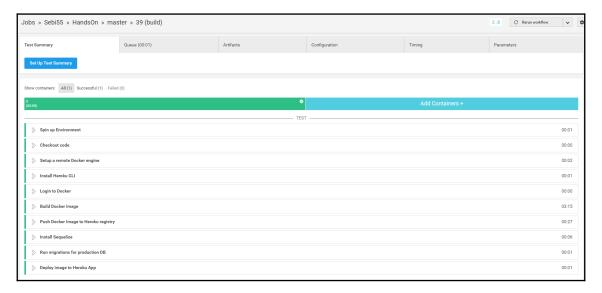
As you can see in the preceding screenshot, all of the steps of our <code>config.yml</code> file are listed with their names and were successfully executed. Your application should be running now. The image was pushed to the Heroku image registry, which directly deployed the latest version of our image to the Heroku app.
