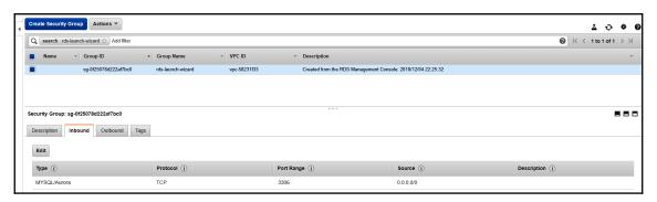
In the preceding screenshot, you can see how the security groups for your new database should look. At the bottom of the window, inside of the small view, select the **Inbound** tab. There, you will be able to insert the IP that is allowed to access the database. If you insert the 0.0.0.0 IP, it will allow any remote IP to access the database. This is not a recommended database setup for production use, but it makes it easier to test it with multiple environments in developmental use.
