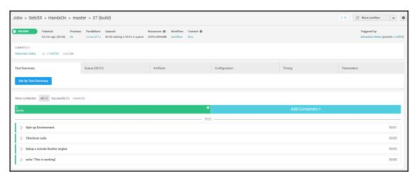
In the preceding screenshot, each step is represented in a separate row, at the bottom of the window. You can expand each row to see the logs that printed while executing the specific command shown in the current row. The preceding screenshot shows that the job has been successful.
