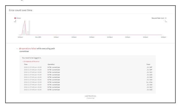
The first chart shows the number of errors over a timeline. Under the graph, you can see each error with a timestamp and the stack trace. You can follow the link to see the trace in detail, with the location of the error. If you paid for the Team plan, you can also set alerts when the number of errors increases or the latency time goes up. You can find these alerts under the **Integrations** tab.
