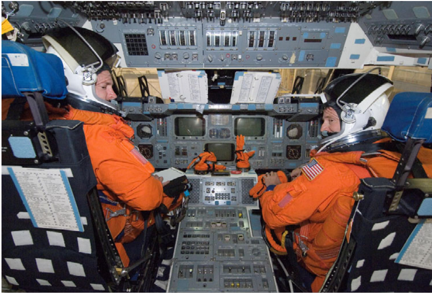
Figure 3.2 A space shuttle simulator has realistic joysticks and screens to simulate the outside world. (Photo courtesy of NASA)
