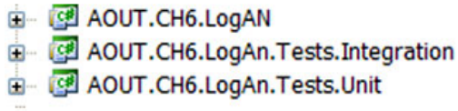
Figure 6.2 The unit-testing and integration projects are unique for the LogAn project and have different namespaces.
