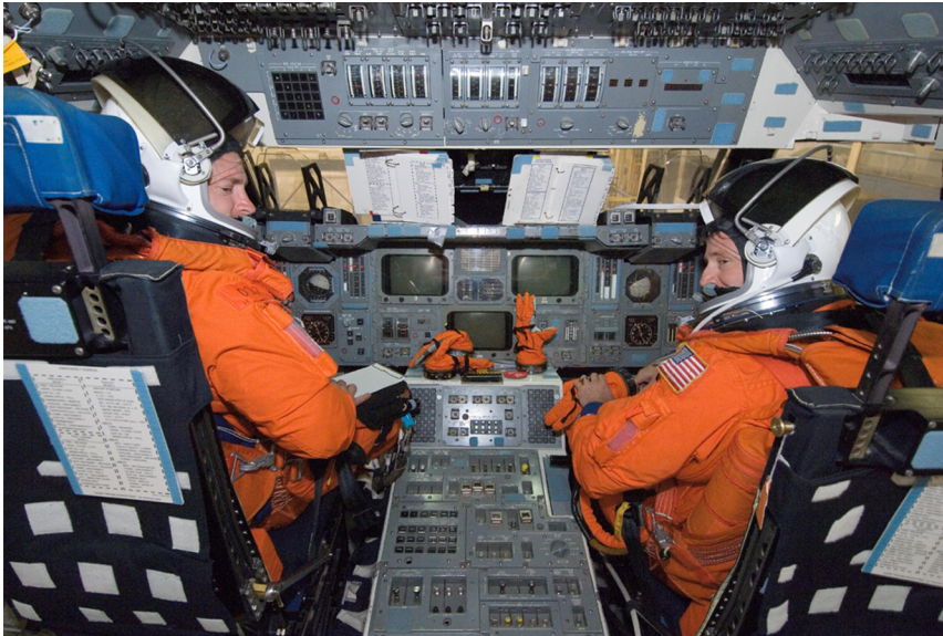
Figure 3.2 A space shuttle simulator with realistic joysticks and screens to simulate the outside world. (Photo courtesy of NASA)
