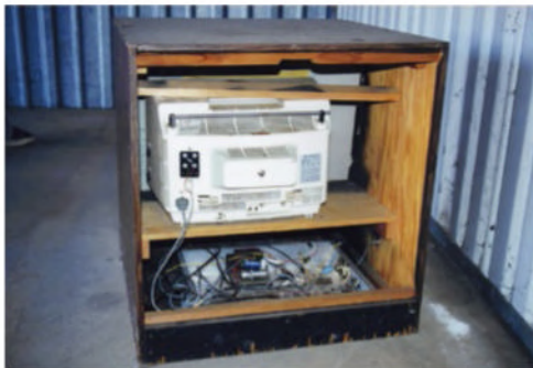
» The inside of the first Pong . A simple wooden shelf with a standard 13-inch black-and-white Hitachi that Ted picked up. The prototype Pong sits in the bottom of the cabinet.
