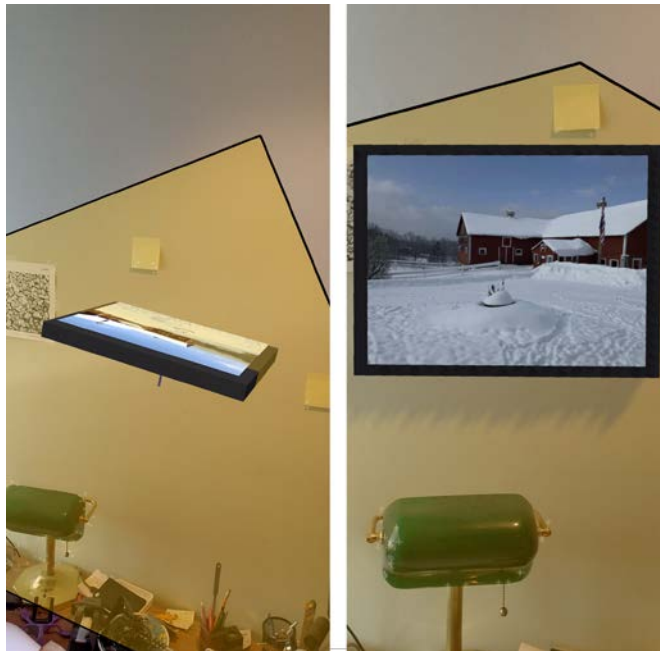
Figure 6.11 – Placing an object on the wall (left) and correcting for surface normal and upright (right)
