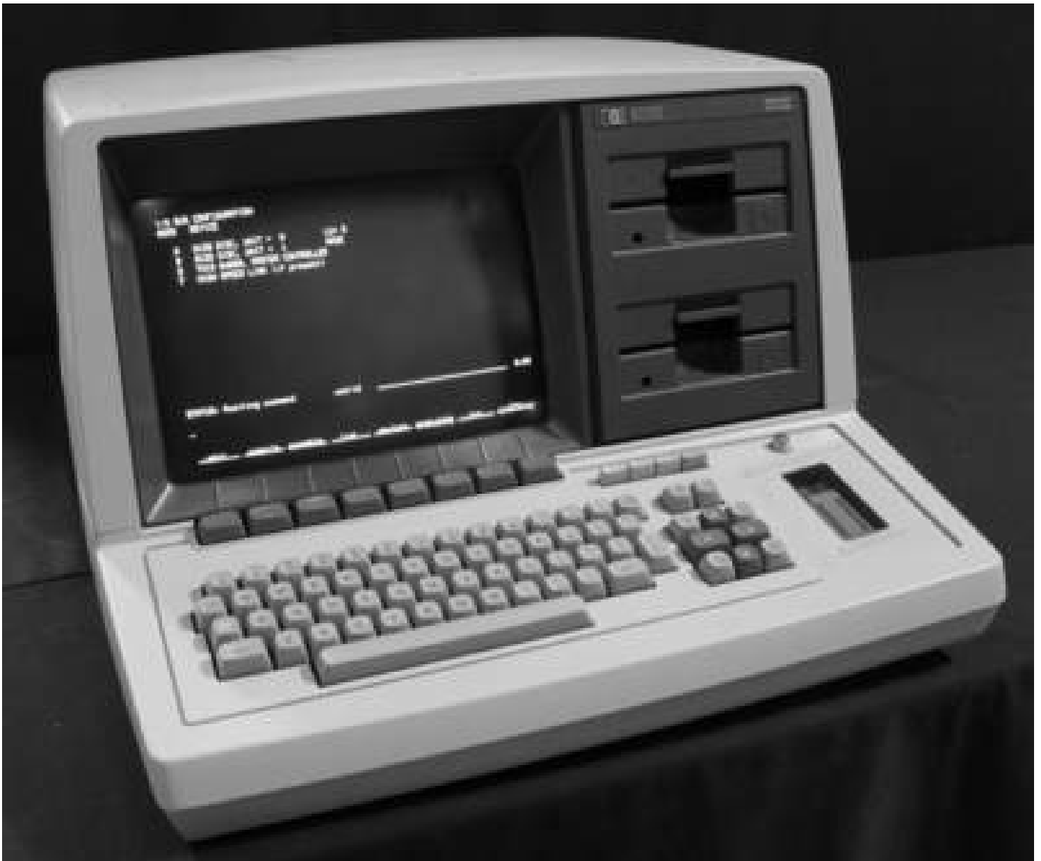
Photo of a 64100A kindly supplied by Jon Johnston of the HP Computer Museum, Australia. The slot to the right of the keyboard is the PROM programmer. www.hpmuseum.net
