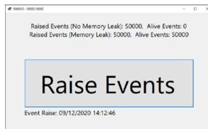
Figure 4.10 – Our Windows Forms application showing 50,000 alive events, indicating we have a memory leak
