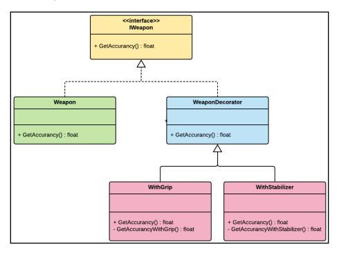
Figure 12.1 - UML diagram of the Decorator pattern
