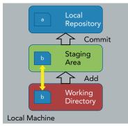
**FIGURE 6-13:** Diffing from the working directory with a version in the staging area
