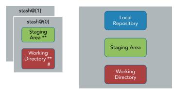
FIGURE 11-4: After stashing, including the untracked file
