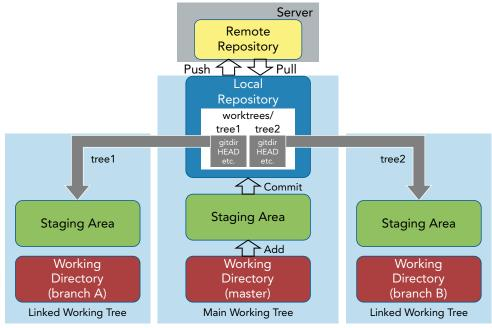
FIGURE 14-1: Illustration of multiple working trees
