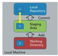
**FIGURE 6-14:** Diffing starting at the staging area
