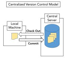
**FIGURE 2-1:** A traditional centralized version control model
