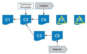
FIGURE 9-10: Applying deltas on the destination tip
