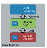
**FIGURE 6-3:** Version *a* of the file is staged.
