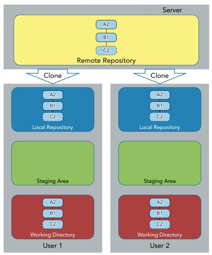
FIGURE 13-3: Two users with the same cloned contents
