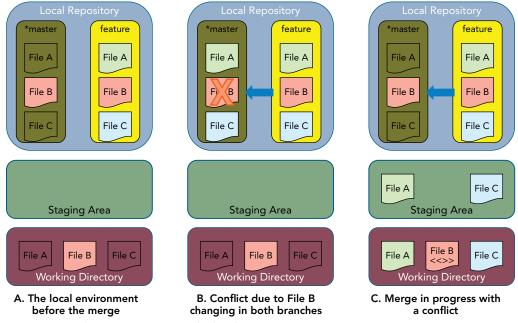
FIGURE 9-14: The merge process in the local environment
