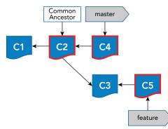
FIGURE 9-4: The three points considered for the three-way merge
