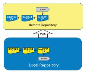
FIGURE 12-6: After a push to the remote repository
