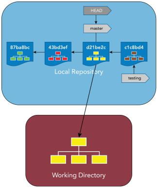
FIGURE 8-9: Git checkout master (again)
