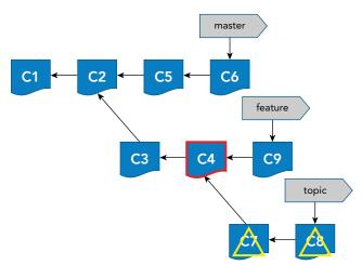
FIGURE 9-28: Computing the deltas to rebase
