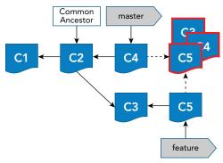
FIGURE 9-5: The three-way merge process
