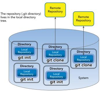
FIGURE 5-3: Working with multiple repositories
