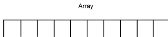
Figure 5.2: Array elements are stored in contiguous memory
