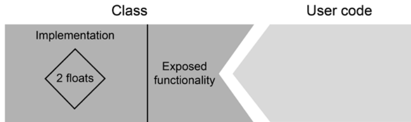
Figure 2.1: The class exposes functionality that the user code uses directly, hiding the fact that it is implemented with two floats
