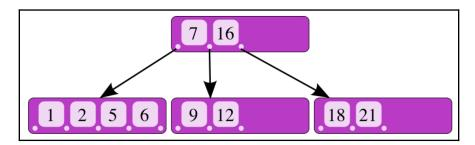
In the preceding diagram, we have a parent node with the values 7 and 16, pointing to three child nodes.
