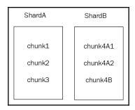
As you can see from the preceding diagram, MongoDB will try to split >64 MB chunks in half in terms of size. The bounds between the two resulting chunks may be completely uneven if our data distribution is uneven to begin with. MongoDB can split chunks into smaller ones, but cannot merge them automatically. We need to manually merge chunks, a delicate and operationally expensive procedure.
