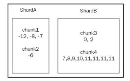
In this case, we observe that *chunk4* has more items than any other chunk. MongoDB will first split *chunk4* into two new chunks, attempting to keep the size of each chunk under a certain threshold (64 MB, by default).
