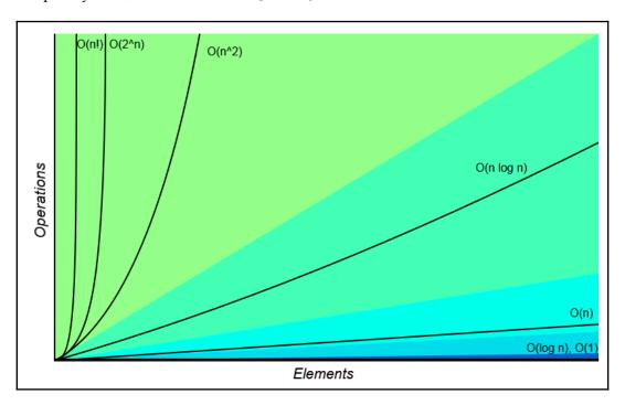
In this diagram, you can see logarithmic time performance as a flat line, parallel to the x axis of the diagram. As the number of elements increases, constant time (O(n)) algorithms perform worse, whereas quadratic time algorithms ( $O(n^2)$ ) go off the chart. For an algorithm that we rely on to get our data back to us as quickly as possible, time performance is of the utmost importance.
