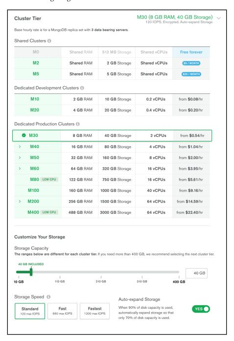
This is similar to how we will select servers in EC2 or Microsoft Azure. The main point to note is that we can select custom IOPS (the number of I/O operations per second) performance, and that we should select the **Auto-expand Storage** option to avoid running out of disk capacity. Together with this option, it's always useful to keep an eye on storage allocation to avoid excessive charges at the end of a billing cycle.
